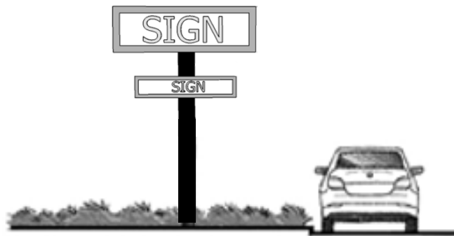
18 A pylon sign with two (2) sign areas
